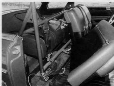
Above: A Spanish-speaking Dennis the Menace adorned the hood as a good-luck mascot. Below: Driver and navigator were securely belted into Lincoln's slick seats. Huge fuel tank occupies rear seat area.
